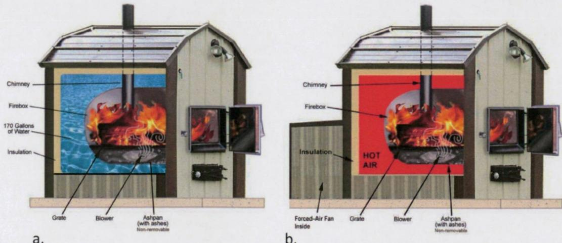
Fig. 4. Outdoor wood boilers (OWBs) a. hydronic [32] b. forced hot air [33].
