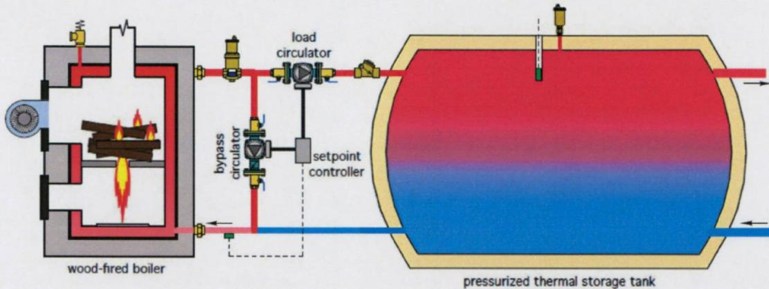
Fig. 3. Advanced wood-fired boiler with thermal storage [29] (Courtesy of John Siegenthaler P.E.).
